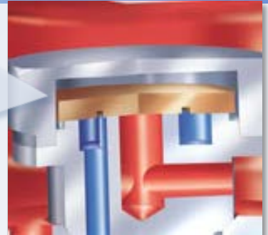
Integral non-return function for high performance
