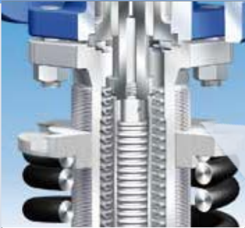
Exact and easy adjustment, diameter independent spring ranges
