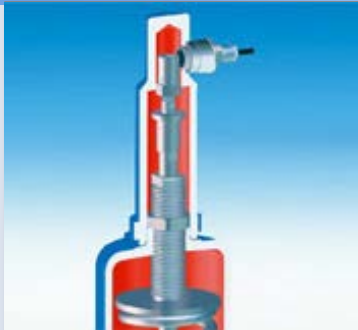
Integrated proximity switch (feedback signal returned to control room for example)
