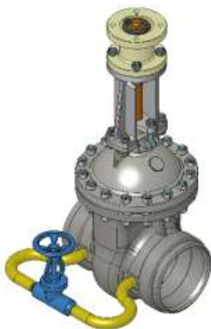
Bypass system with one isolating valve
